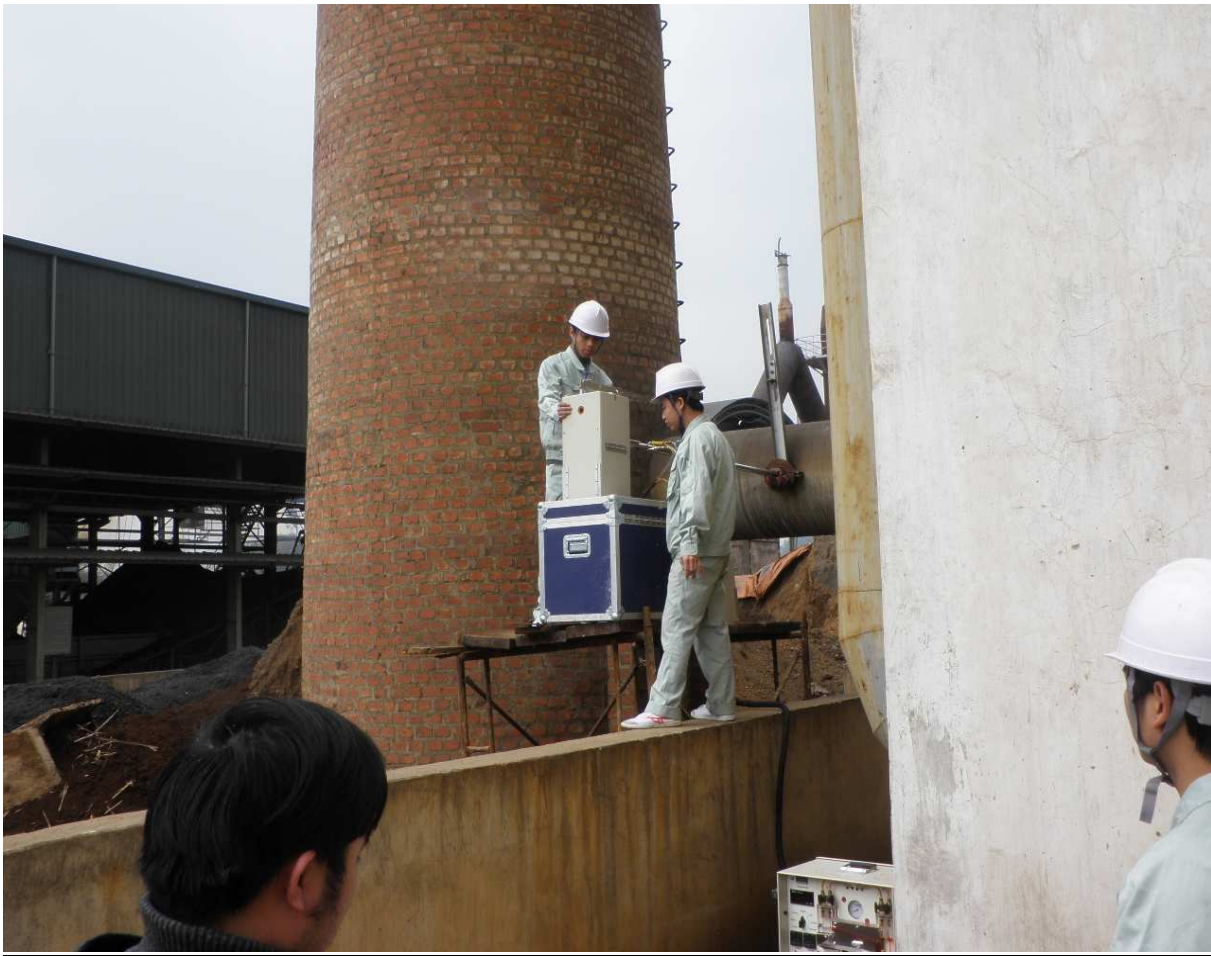
Technicians of the Dioxin Laboratory collecting stack samples in a factory
