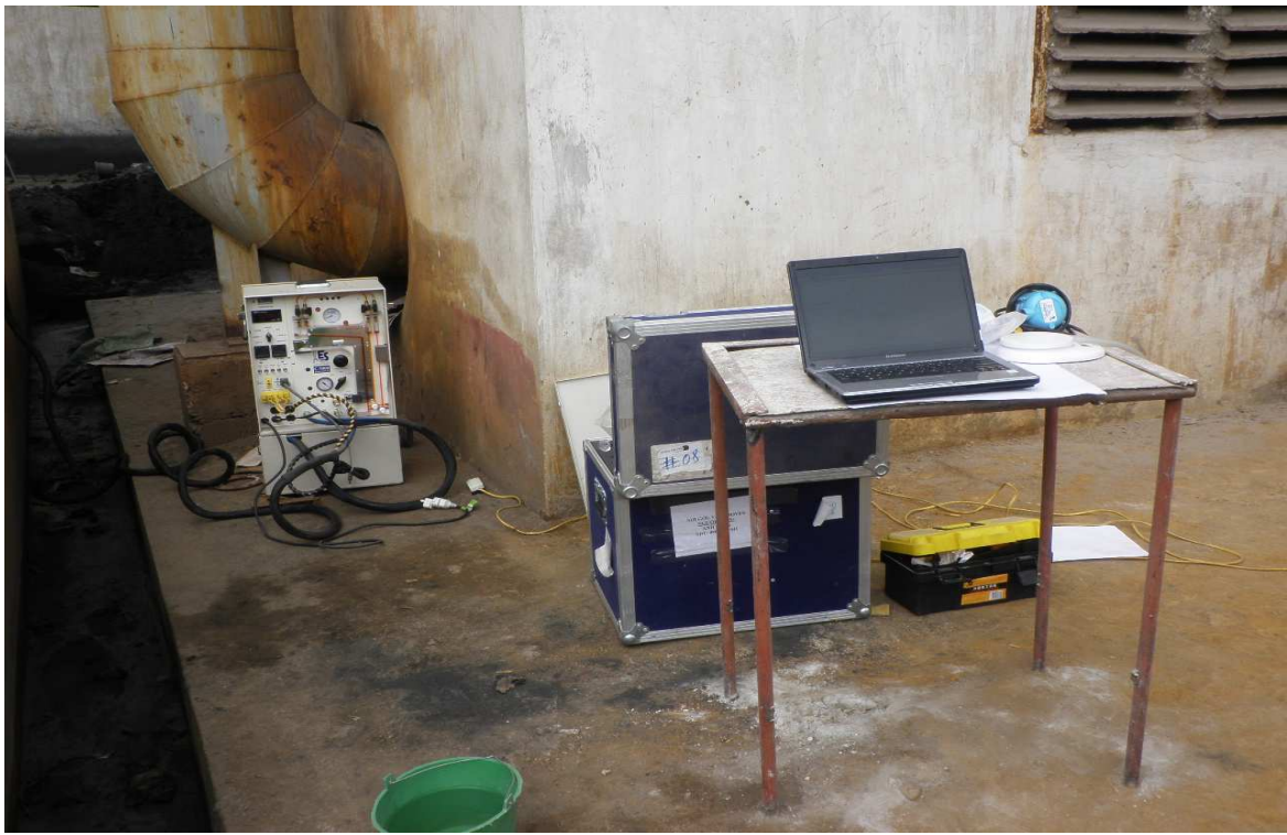
Measurement equipment for emissions provided by the project
